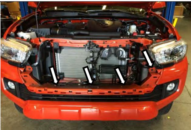
4. Remove the bumper, by releasing the clips along the top return and below the head light. If there are fog lights fitted be sure to unclip the harness.
