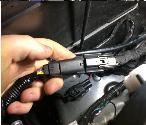
43. Disconnect the 6-pin connector from the back of the headlight on the left side of the vehicle. Plug this connector into the corresponding side of the harness headlight connectors.
