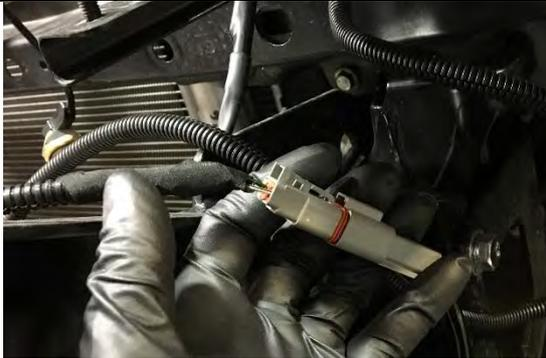
46. Connect the fog harness using the 2-pin Deutsch connectors.
