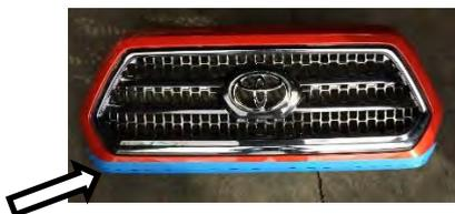
23. Using an oscillating multi-tool carefully cut the bumper ends (LH & RH) and the grille along marked lines.
