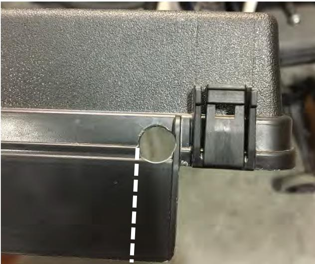
35. Drill a  $\varnothing 10\text{mm}$  hole in the right side of the fuse box cover right next to the edge as shown. Trim parallel to the edge, straight down.
