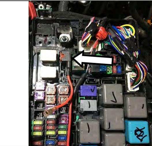
34. Find the fuse tap included in the harness bag and plug the removed fuse into the lower slot of the tap.
