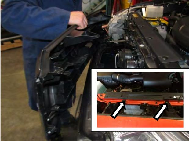
2. If fitted, remove licence plate from bumper. Remove the two top screws on the grille.
