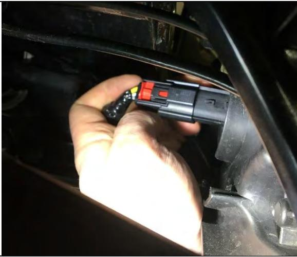
44. Insert other side of the 6-pin connector into the back of the headlight.
