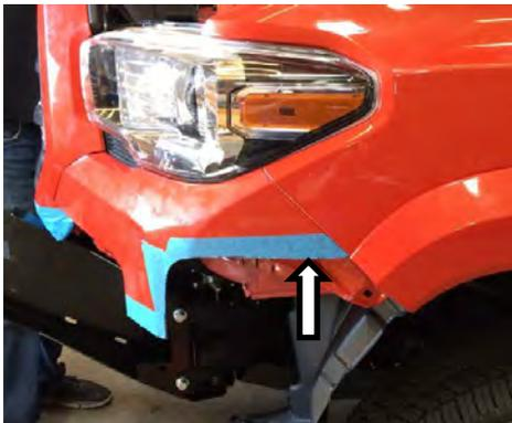
26. Using the refitted cut bumper end as a guide mark the bumper retaining bracket.
