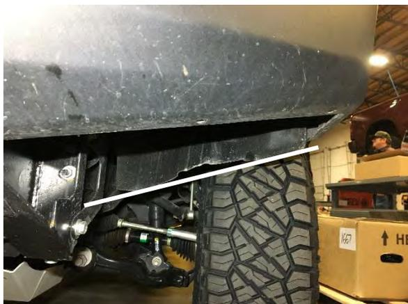
76. Once under wing panel is fitted, mark a line approximately 5-10mm above the wing panel. Cut the wheel well liner using an oscillating multi-tool and tuck behind the rear lip of the wing under panel. Repeat for other side.
