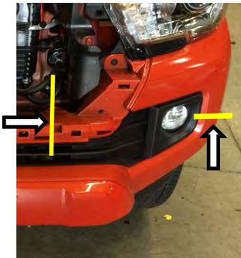
22. Cut the corners off as indicated in the picture using an oscillating multi-tool.
