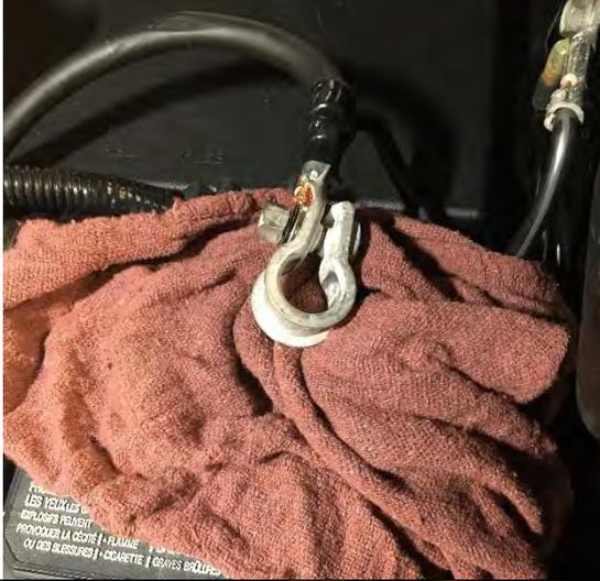
1. Disconnect the battery's main ground from the battery and push the cable to the side. A rag or other cover can be used to ensure the wire does not touch the battery terminal.
