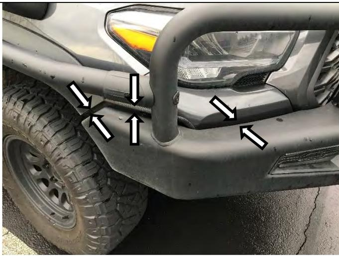
59. Align bull bar so there is a 15-18mm gap from top of wings to underside of flares and an even 10mm minimum gap to vehicle including periphery under headlights, and then tighten all bolts.
