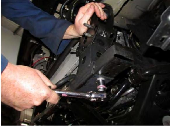
10. Remove lower bolts on cross member and remove cross member extensions both sides as shown and discard.
