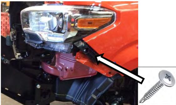
31. Refit the cut bumper retainer. Only use the top bolt to hold the bracket in place.
