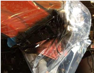
30. Using a black spray can paint the panel. Allow to dry before removing tape. Repeat for other side.
