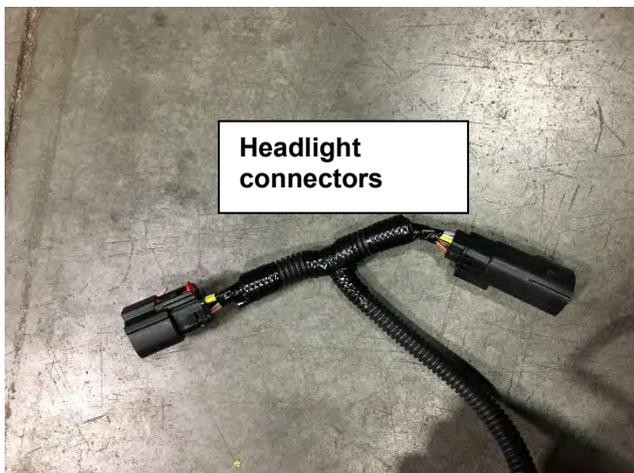
39. Identify 6-pin headlight connectors, Deutsch 6-pin, and Deutsch 2-pin connectors.
