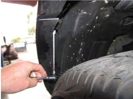
6. Remove the two front wheel arch bolts. Pull bumper ends out and away from vehicle to release them from clips. You will also need to unclip the wheel arch flare. Remove bumper and place on work stand front face up.
